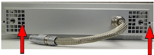
13. Locate the center hole in each end of the lamp housing cover.
