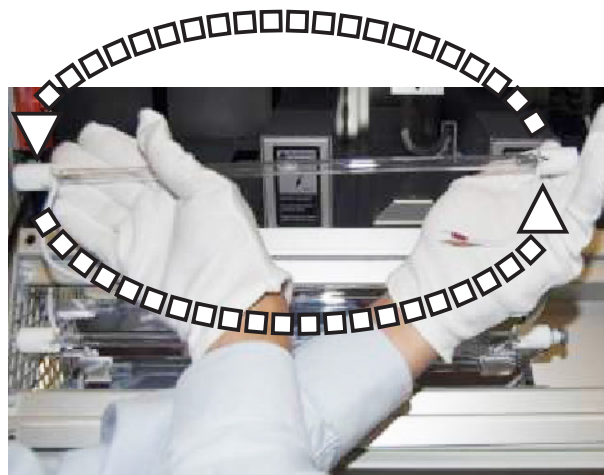
Figure 15.5b: Swap Ends to Reverse the Lamp and Reinstall
