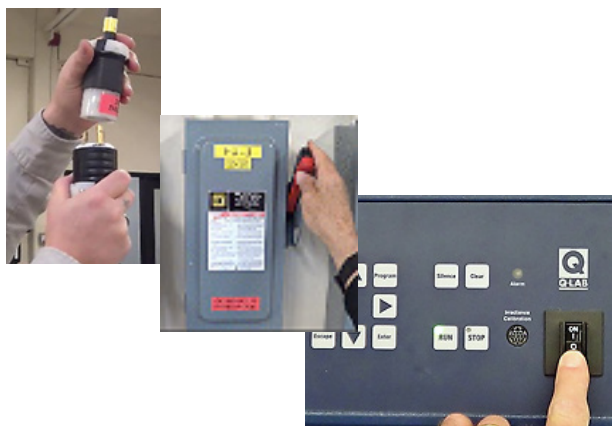
28. Reconnect Power. Power ON. Xe-1 power ON.
