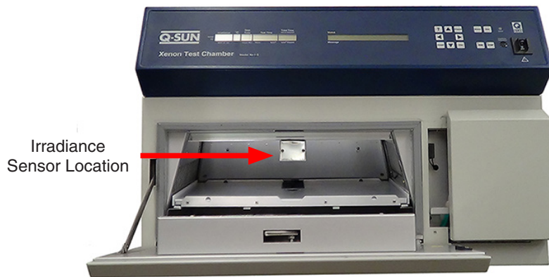
Figure 7.3a: Xe-1 Irradiance sensor located on rear chamber wall (behind shield).
