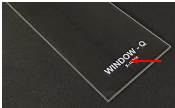
Figure 10.2a: Optical Filter Type Etched into Filter
