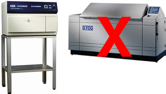
Figure 4.2a: Do not install testers in a room with corrosion chambers.
