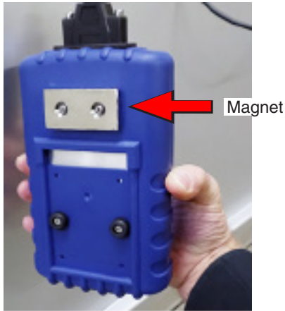
9. The UC1 unit has a magnet on the back.
