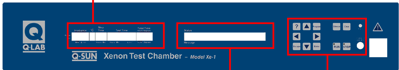
Figure 9.2b: 10.2b: Xe-1 Full Control Panel
