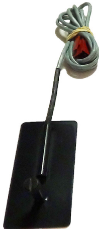
Figure 8.1a: Uninsulated black panel temperature sensor.
