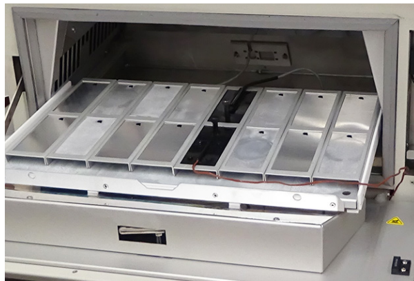
14. Place Q-SUN and UC202 black panels in holders on the tray with specimens in holders.
