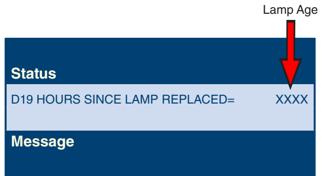
Figure 14.1b: D19 shows the number of hours since the lamp was last replaced
