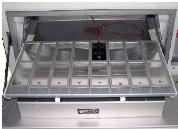
Figure 10.3f: Panel Holder Kit (Part Number X-10113-K) with (8) Panel Holders Holding (15) 50×100 mm (2×4") Specimens and (1) Black Panel
