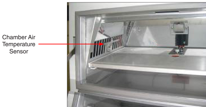
Figure 8.2: Optional CAT sensor location in the test chamber.
