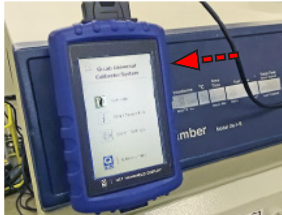
10. When performing calibrations, the UC1 can be held in place by the magnetic mounting strip.
