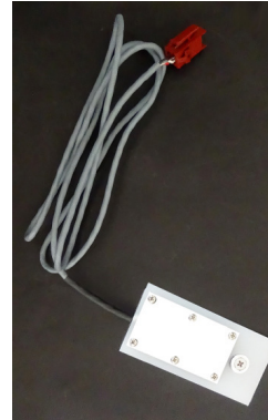
Figure 8.1e: Insulated white panel temperature sensor.
