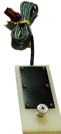
Figure 8.1b: Insulated black panel temperature sensor.
