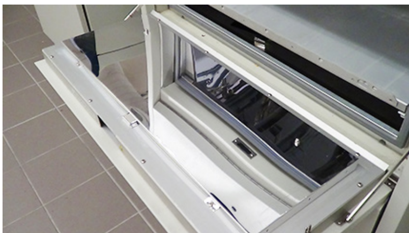
Figure 14.5c: Clean Reflector - OK
