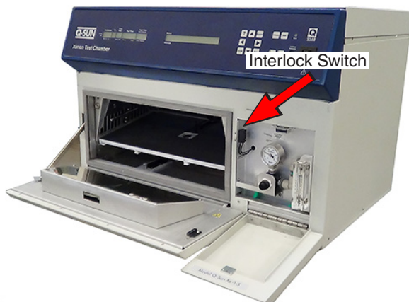
Figure 2d: Basic model tester chamber door interlock switch location (test chamber and plumbing access door open).
