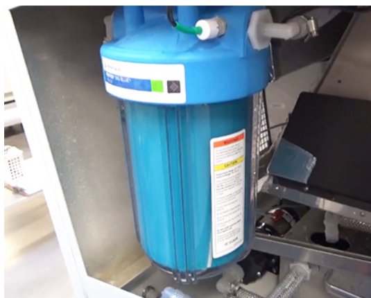
28. Check for water leaks around the housing cap. If any leaks, re-tighten the housing.
