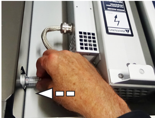
26. Reconnect the power wire.
