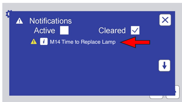
Figure 16.1a: M14 Time to Replace Lamp displayed on the Notifications Screen.
