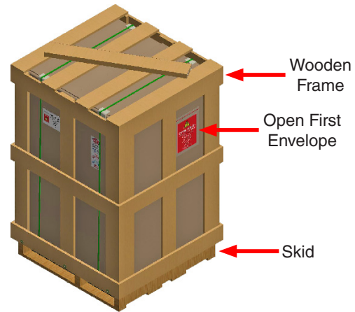
Figure 5.3b: This packaging has a carton surrounded by a wooden frame fastened to a wooden skid.
