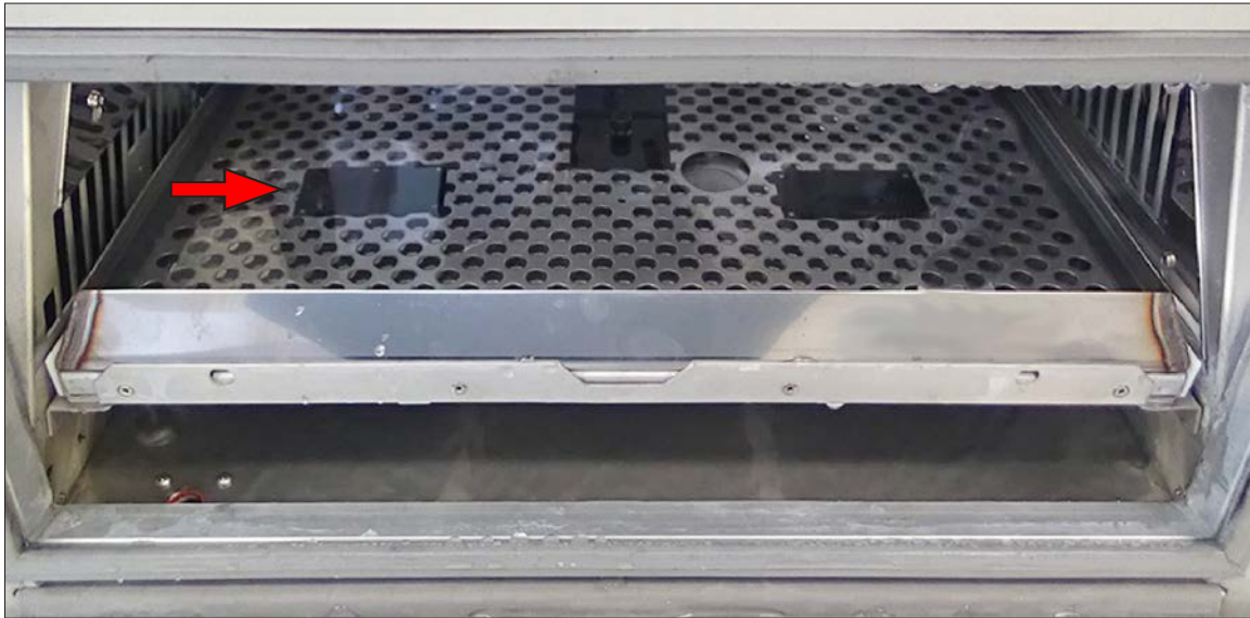
Figure 12.5s: Place specimens on the mesh insert.
