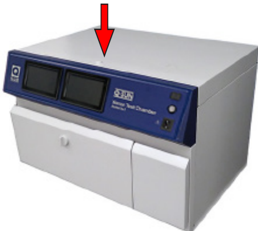
5. Use a flat blade screwdriver to open the latch on the lamp door.
