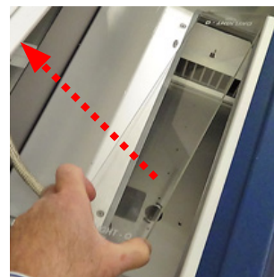
Figure 12.4d: Remove the UV filter.
