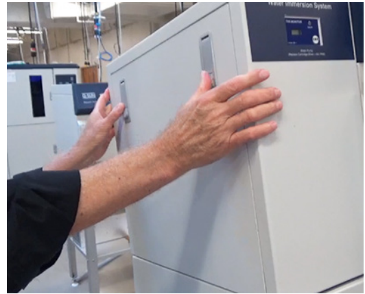
30. Close the access panel latches.
