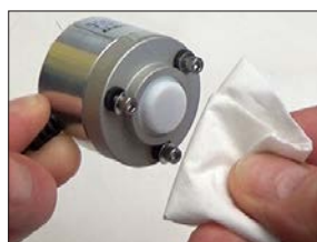
Figure 13.1e: Clean the sensor face with 99% isopropyl alcohol and a soft cloth.
