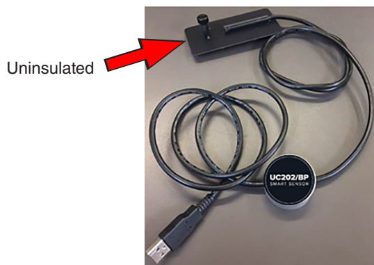
Figure 13.2a: UC202/BP Temperature Smart Sensor with Uninsulated Black Panel (Black Panel)
