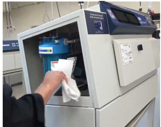
8. Place paper towels in the Xe-1-WE below the filter housing to absorb any spilled water.
