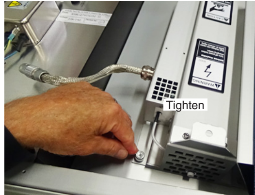
25. Tighten the captive stud.
