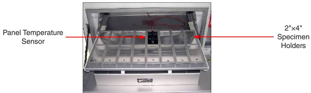
Figure 10.1f: Correct location of the Xe-1-SE, Xe-1-BCE and Xe-1-SCE panel temperature sensor.
