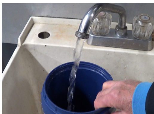
5. Fill an insulated container with water of approximately the same temperature to which the chamber air temperature will be set.
