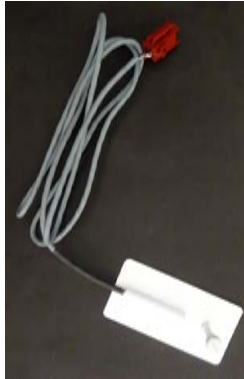
Figure 10.1d: Uninsulated white panel temperature sensor.
