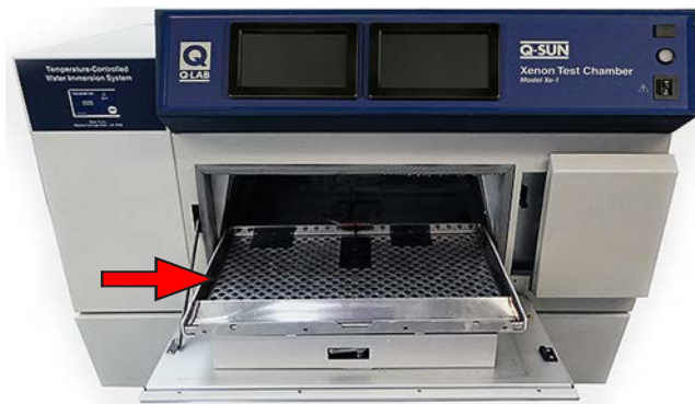
Figure 12.5b: Xe-1-WE with ponding tray mounted on specimen tray.
