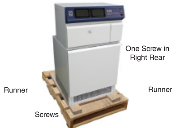
16. Screws (2 each side) attach runners to skid.
