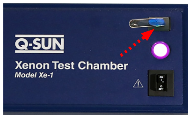
Figure 16.7b: Connect the drive to the USB port on the Q-SUN control panel.
