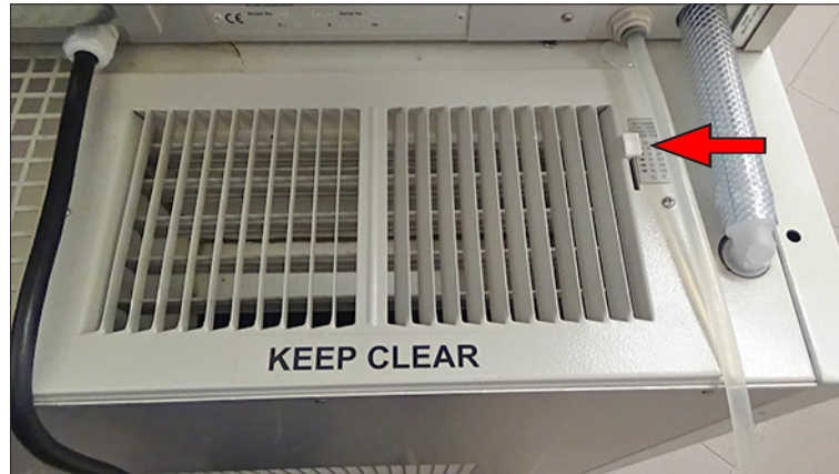
Figure 12.3d: Xe-1-BCE and Xe-1-SCE damper adjustment.
