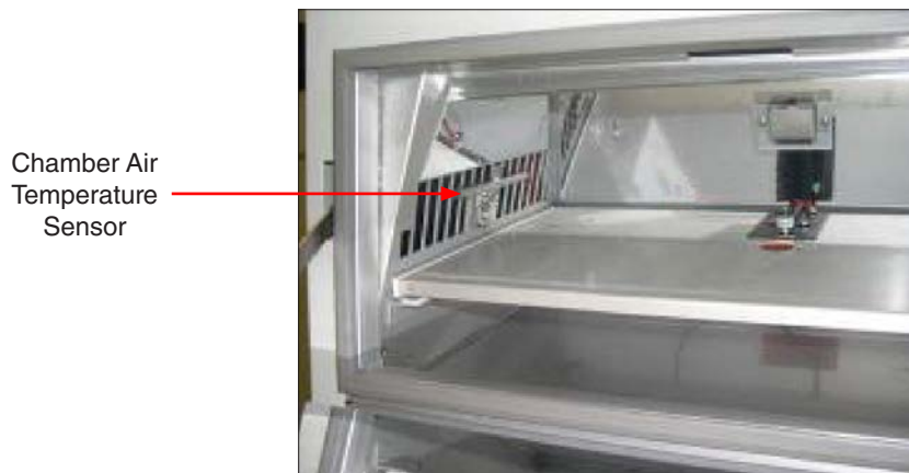
Figure 10.2: Chamber air temperature sensor location in Xe-1-BCE and Xe-1-SCE test chambers.
