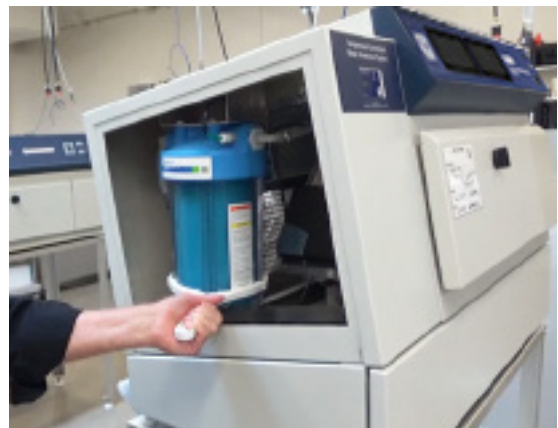
10. Place the wrench on the housing.
