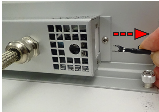
16. Disconnect wire at opposite end of lamp housing cover.
