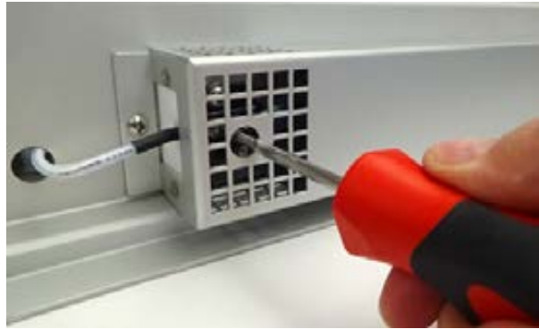
14. Insert a Phillips screwdriver in the center hole. Loosen the screw.
