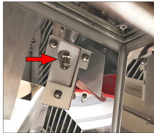
Figure 16.6b: Interior of chamber showing right-side spray nozzle.
