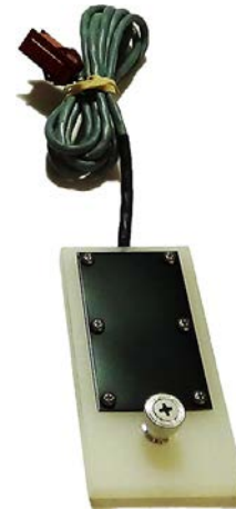
Figure 10.1b: Insulated black panel temperature sensor.
