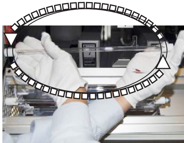
Figure 17.3b: Swap ends to reverse the lamp and reinstall.
