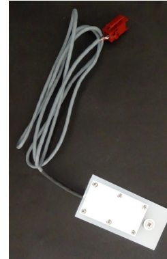
Figure 10.1e: Insulated white panel temperature sensor.
