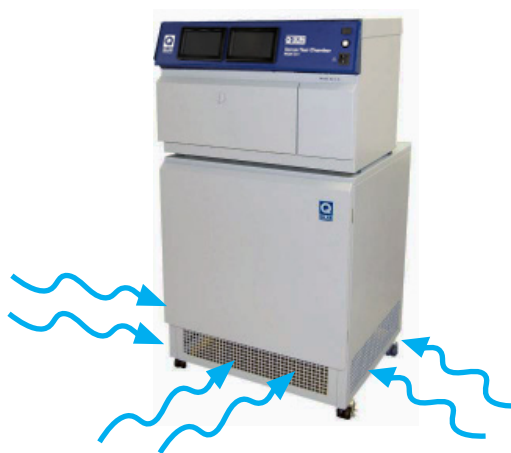
Figure 6.4c: Q-SUN Xe-1-BCE and Xe-1-SCE chiller cooling air intake areas.
