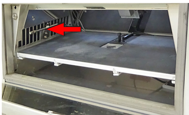
3. Locate the air temperature sensor mounted on the grill in the left side of the chamber.
