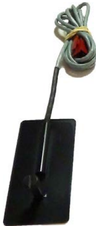
Figure 10.1a: Uninsulated black panel temperature sensor.
