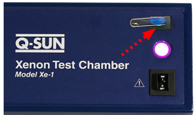
Figure 14.3b: Connect the drive to the USB port on the Q-SUN control panel.
