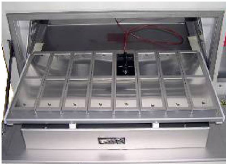
Figure 12.5g: Panel holder kit (X-10113-K) with eight (8) panel holders holding fifteen (15) 50×100 mm (2"×4") specimens and one (1) black panel.
