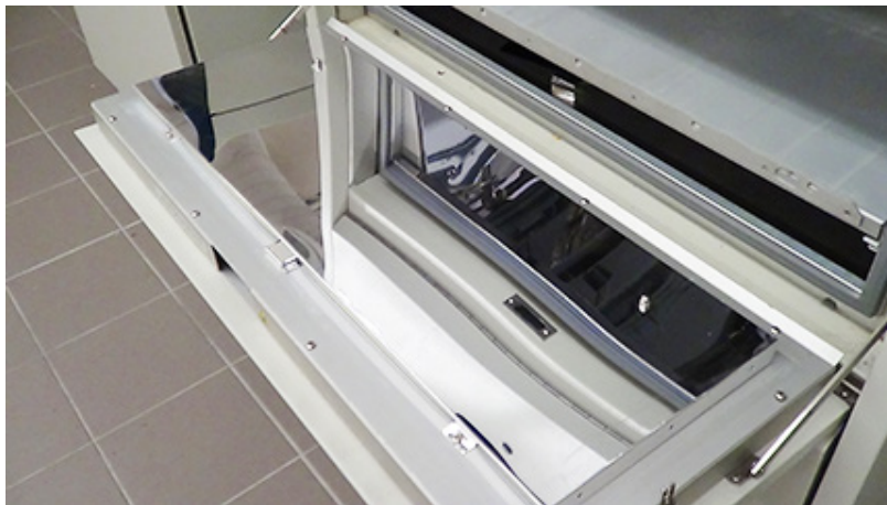
Figure 16.6d: Clean Reflector - OK
