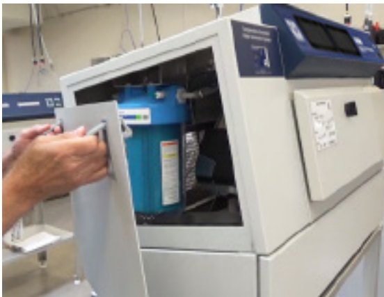
7. Remove the access panel. Set aside.
