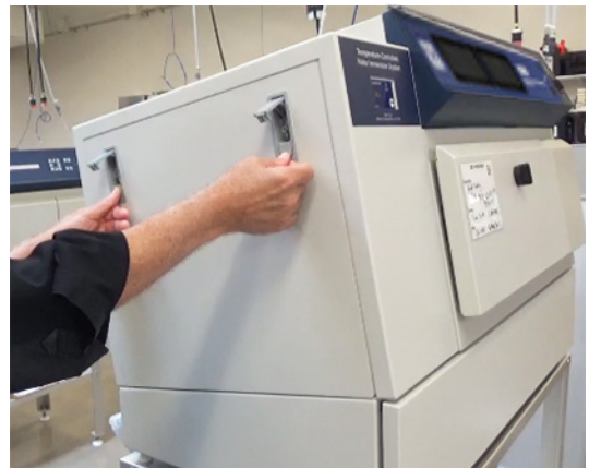
6. Open the latches on the left side access panel.
