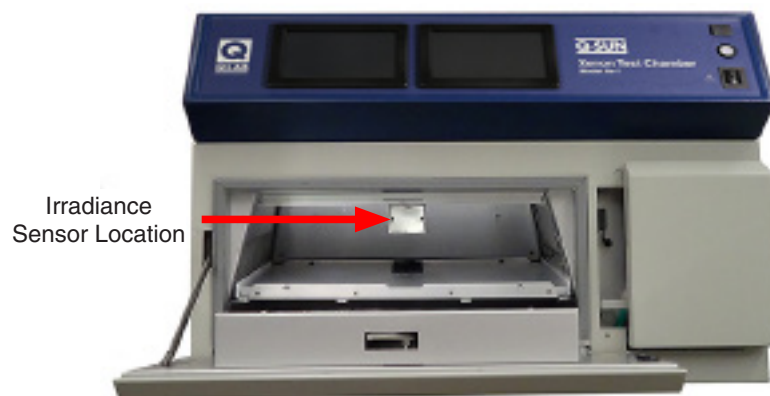
Figure 7.3a: Xe-1 Irradiance sensor located on rear chamber wall (behind shield).
