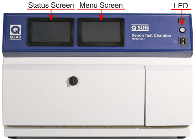
Figure 11.1a: Touch-screens and LED location.
