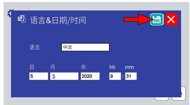
Figure 11.7l: All text on both screens will be in the selected language. Touch the save icon to save the selection.
